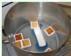
**Cleaning:** Soaking 15 min in a solution of hot (50°C) alkaline detergent followed by brushing for approx. 30 sec and rinsing with hot water
