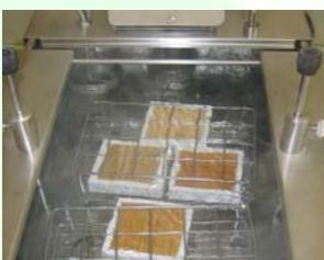
**Heat desinfection:** 80°C, 5 min and 65°C, 15 min, respectively
