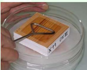
**Contamination** with *Listeria monocytogenes* ( $10^5$ - $10^6$  CFU/cm<sup>2</sup>). Thereafter the blocks were stored in a wet chamber at 21-28°C.
